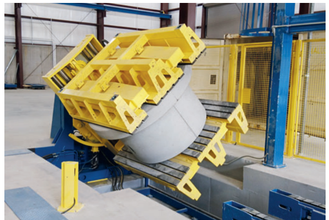
An automated turning station was installed to handle products with base extensions to prevent uplift
